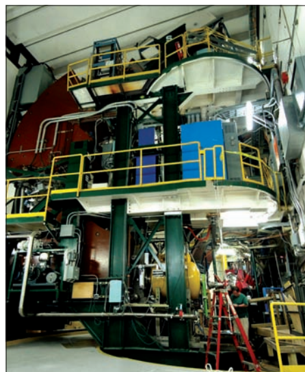
The three-storey S800 spectrograph separates and identifies isotopes after the secondary collision with very high resolution. (Photos courtesy NSCL.)
