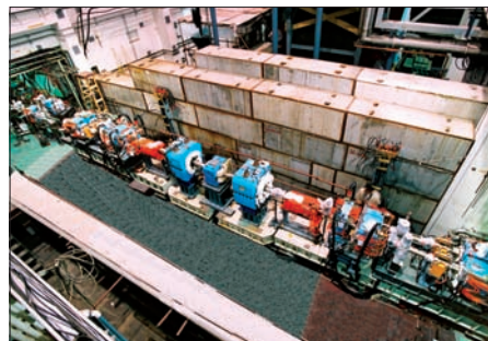
Conventional magnets at BEPCII's interaction region. (Courtesy IHEP, Beijing).
