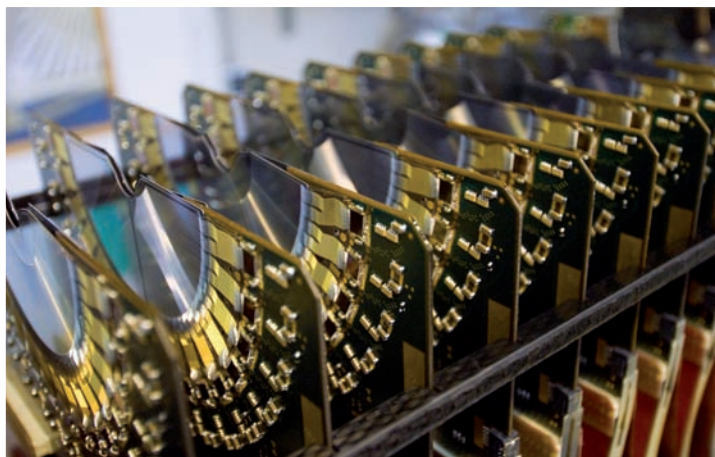
The 42nd and final module for LHCb's vertex locator arrived from Liverpool in March, marking the culmination of 10 years of development. The detector will be placed just 5 mm from the beam line.
