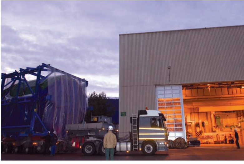
Gently does it: In January, the lorry transporting the time projection chamber for the ALICE experiment took an hour to travel the 200 m from the assembly hall to the access shaft for the underground cavern.
