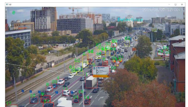
Fig. 9. Congested detected, even image contains ghost tracks and untracked vehicles.
