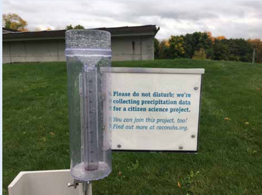
Standard rain gauge. Measurements of rainfall from this gauge are sent to the Community Collaborative Rain, Hail, and Snow Network's database.
