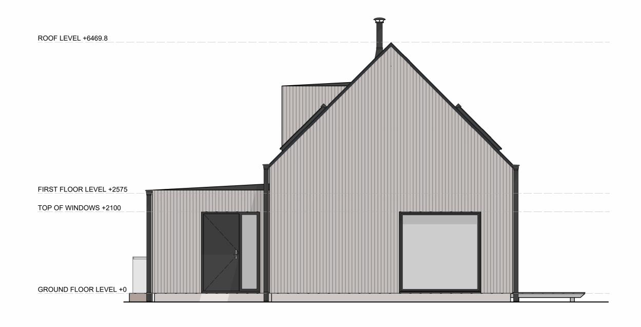
Walls: Vertical Larch, Naturally Weathered Roof: Standing Seam Aluminium, Black Gutters: Exposed Metal Gutters, Coated Black Windows: AluClad windows in Black
