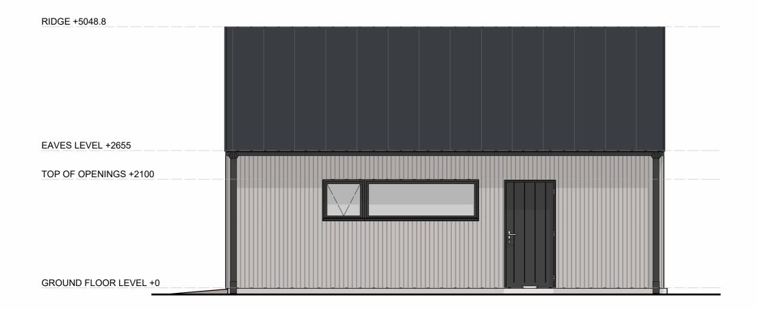
Walls: Vertical Larch, Naturally Weathered Roof: Standing Seam Aluminium, Black Gutters: Exposed Metal Gutters, Coated Black Windows: AluClad windows in Black
