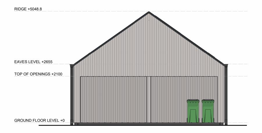
Walls: Vertical Larch, Naturally Weathered Roof: Standing Seam Aluminium, Black Gutters: Exposed Metal Gutters, Coated Black Windows: AluClad windows in Black
