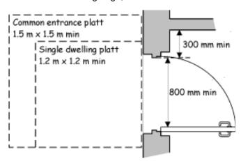
In order to meet the requirements of an accessible threshold, then the threshold should meet the following criteria:
