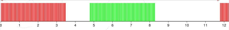
In a closed-burst SAR (CryoSat, S-3, J-CS baseline) transmit and receive are not interleaved and are not continuous. The CryoSat values of N = 64 and PRF = 18 kHz give a burst duration of ~3.5 ms. But the burst-to-burst interval is ~11.8 ms.
