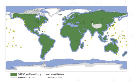
S-3 and J-CS baseline scenarios envision SAR mode (SARM) over coastal zone and conventional (LRM) measurements over open ocean. Since tide gauges are mainly in the coastal mask, we will require inter-calibration of SARM and LRM to bootstrap from coastal gauges to LRM cal.
