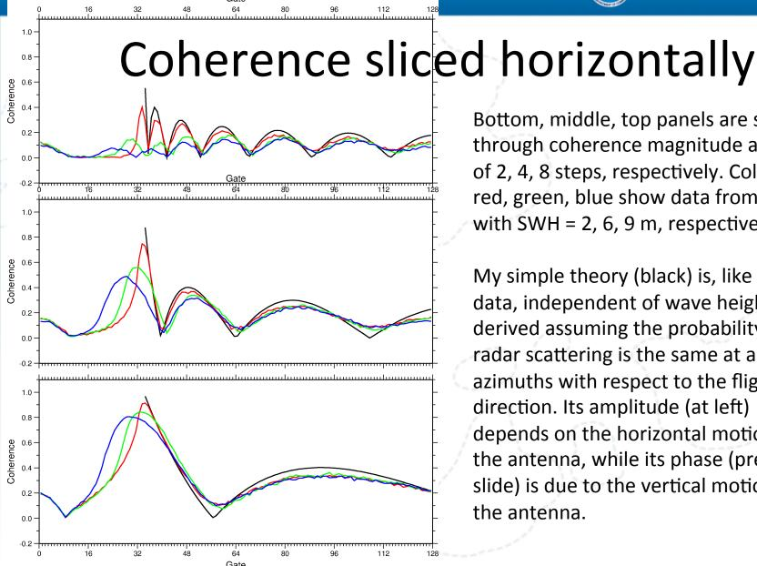
Bottom, middle, top panels are slices through coherence magnitude at lags of 2, 4, 8 steps, respectively. Colors red, green, blue show data from areas with SWH = 2, 6, 9 m, respectively.
