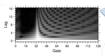
(Biased) Coherence Magnitude,  $\gamma = |C_{k,a}/C_{0,a}|$ Biased: thermal noise only in k=0.
