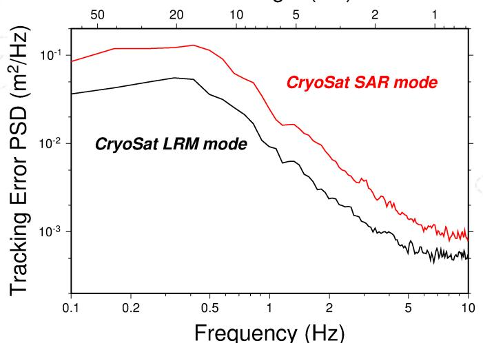
Range gate tracking errors (error in timing the digitizing of the returned radar echoes), expressed as range to the sea surface.
