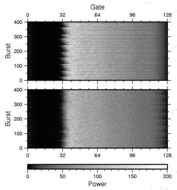
All altimeters, by design, can time the digitizing of received echoes only coarsely. If not corrected, the expected time to nadir jitters by +/- 2 range gates in the waveform.
