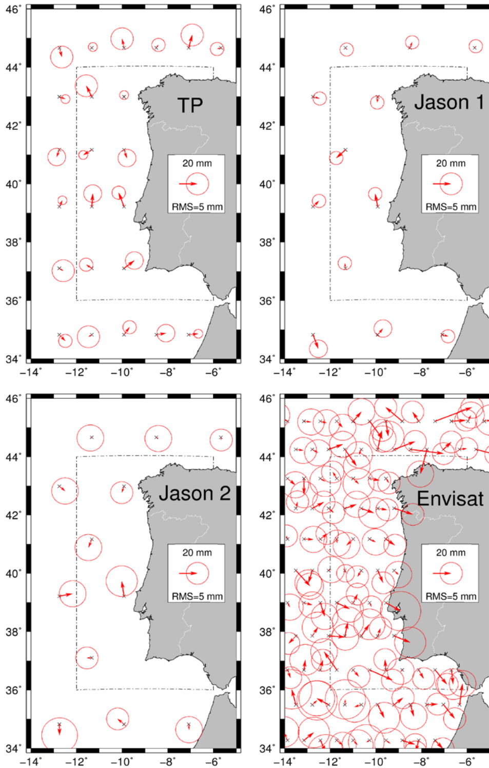
Fig. 10. The results of the residual tidal analysis for harmonic M2 at the cross-over points for the TOPEX/Poseidon, Jason 1 & 2 and Envisat satellite. The arrow length indicates the observed tidal amplitude. The angle with the positive x-axis indicates the observed phase-lag. The error circle indicates the 95% confidence region. The legend shows an observed tide with an amplitude of 20 mm, a zero phase-lag and the 95% confidence region for the case the RMS=5 mm.
