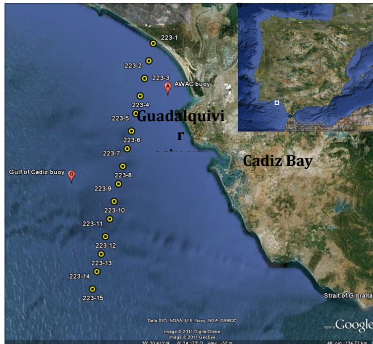
Figure 11: Location of the study area showing ENVISAT track 223 and the AWAC (A) and Gulf of Cadiz (G) coastal buoys. Ground tracks are depicted with yellow dots indicating the position of the 1 Hz measurements (Google Earth copyright).
