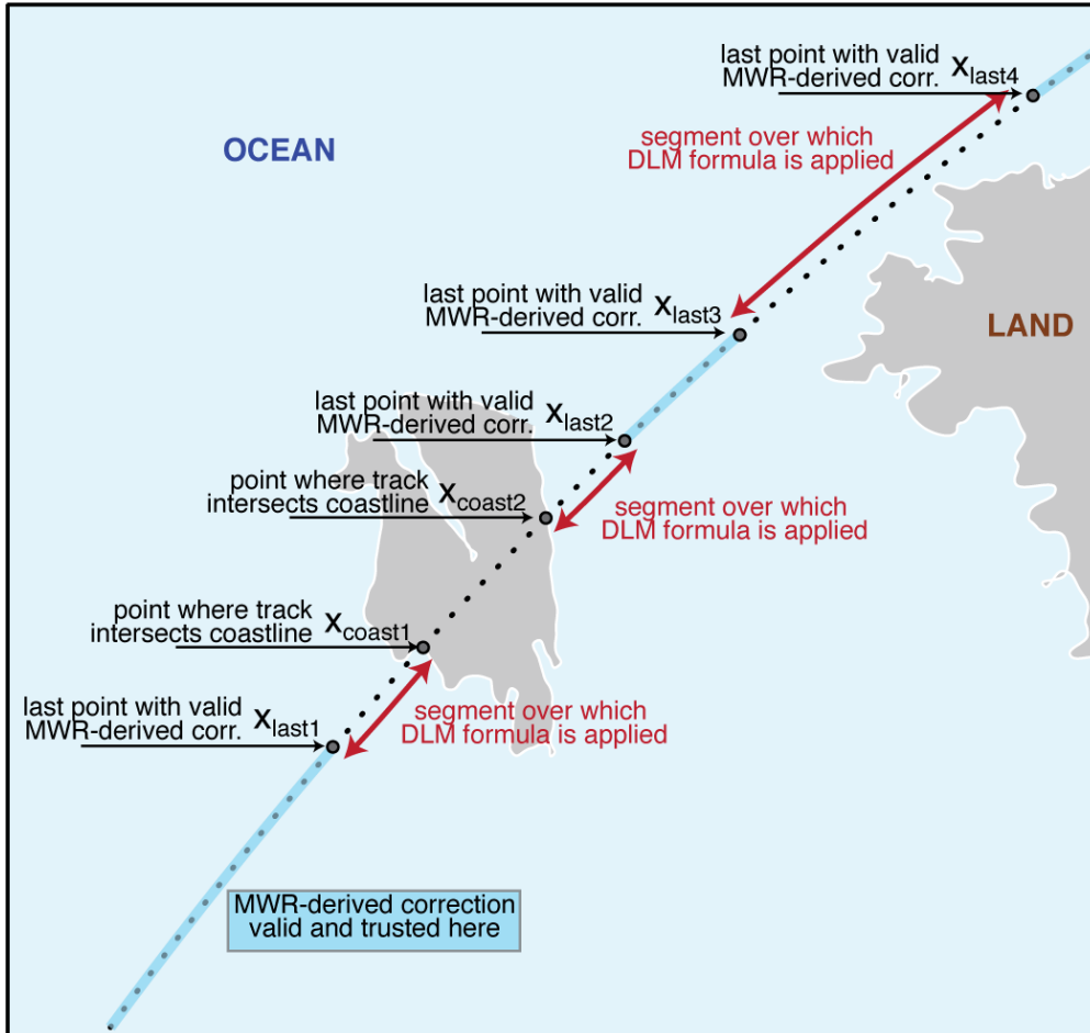
Figure 6: Configuration for short (less than 60km) radiometer data gap or contamination by land located across-track from nadir.
