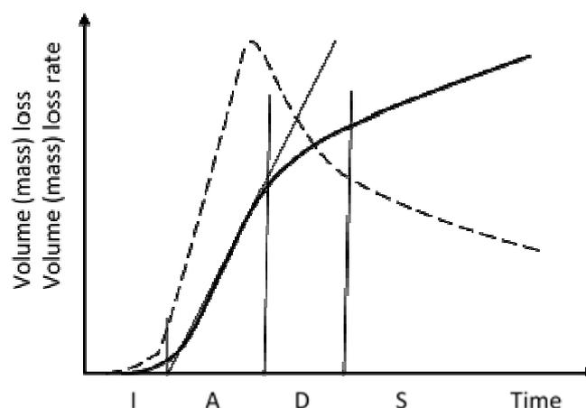
**Fig. 2.** Cavitation curves with showed periods of degradation. solid line – correlation of volume loss in exposure time, dashed line - correlation of volume loss rate in exposure time
