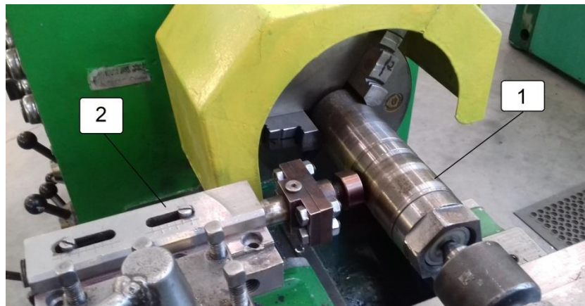
Fig. 3. Test stand for sliding burnishing: 1 – mandrel with samples, 2 – burnishing tool
