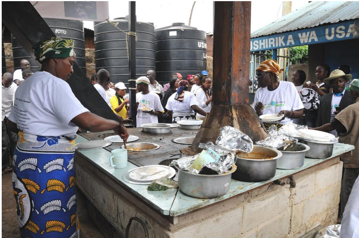
Community cookers in Kibera, Kenya create heat for cooking by burning waste. © Community Cooker Foundation
