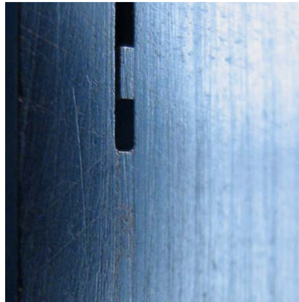
Fig. 1: Vertical cut of a braze sample showing a complete homogeneous filling at the bottom.
