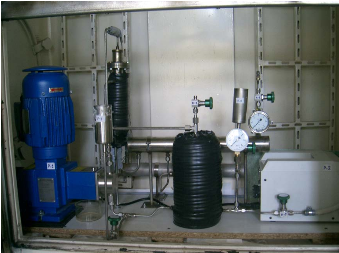
Fig. 1: The experimental rig for endurance tests with 100 Ci kg -1 tritium activity in water.
