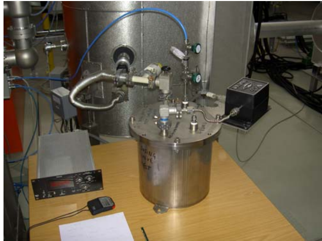
Fig. 2: Calibration set-up for the low flow mass flow controller.
