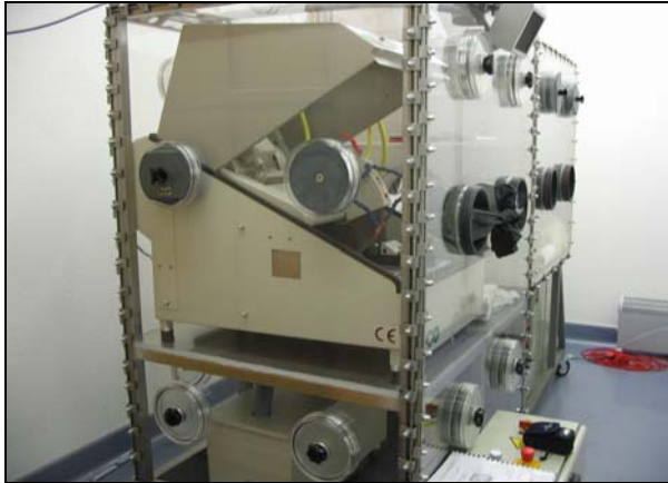
Fig. 1: Glove-box system equipped with Cutting Machine VI-PER 300 A2.
