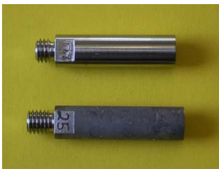
Fig. 11: Cylindrical test samples ( \varnothing = 8 \text{ mm} ) designed for corrosion testing in Pico loop. Top: Bare EUROFER Bottom: Al coated by ECA after heat treatment.
