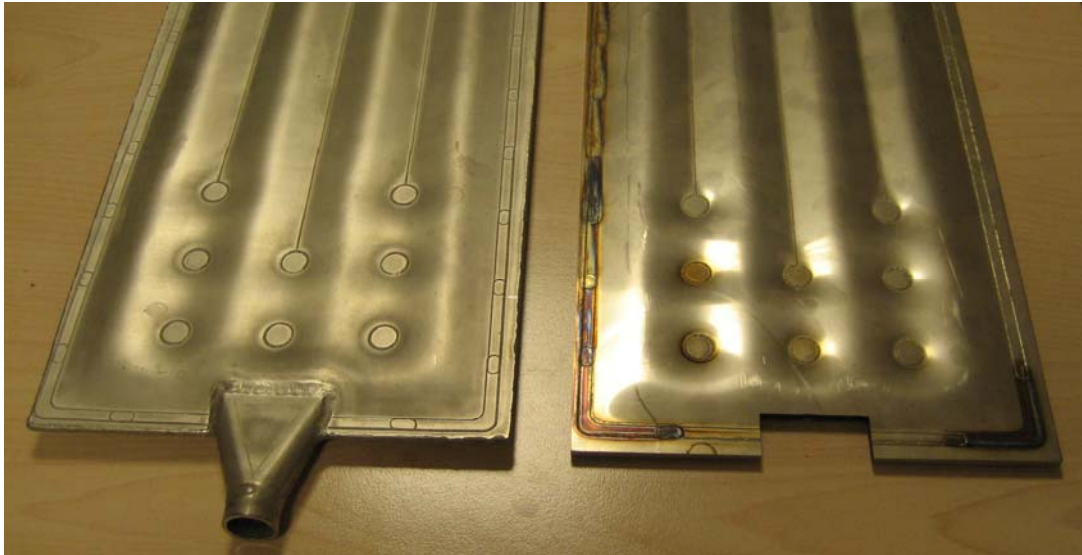
Fig. 2: 4.5 K hydroformed stainless steel panels - pilot production by Omega.
