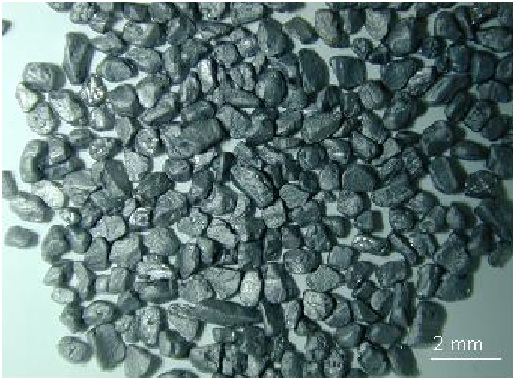
Fig. 1: Be pebbles having average grain size >100\ \mu\text{m} .
