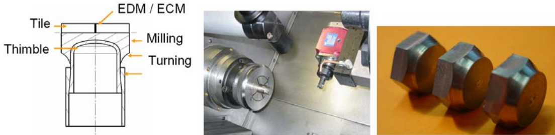
Fig. 10: Left: Different machining types to make the tile. Middle: Machining center. Right: First results.
