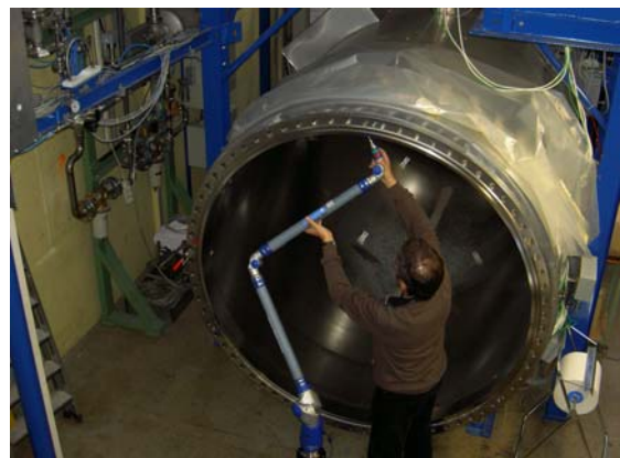
Fig. 3: Roundness measurement activities at the TIMO-2 test vessel flange.
