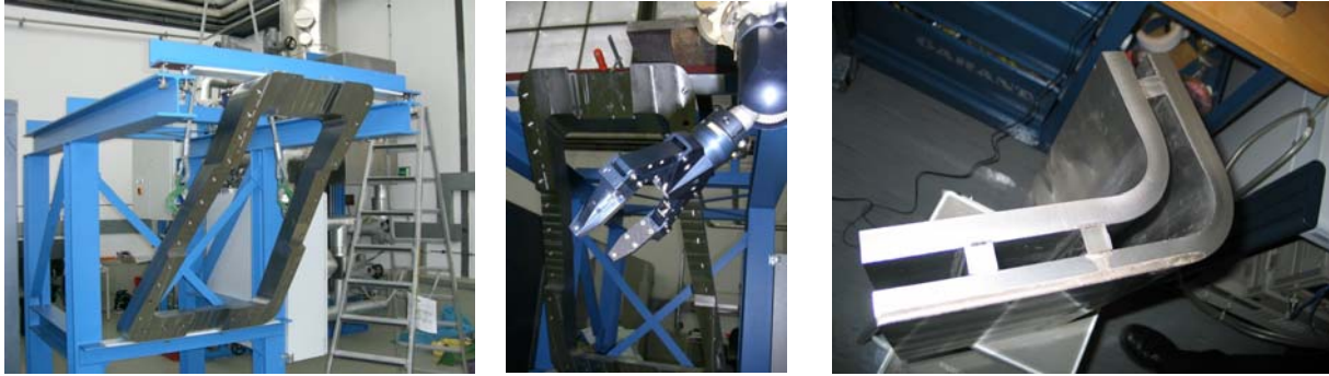
Fig. 3: The Launcher Handling Test Facility (left) with a manipulator arm (middle) and a manufacturing study of the double wall structure (right).
