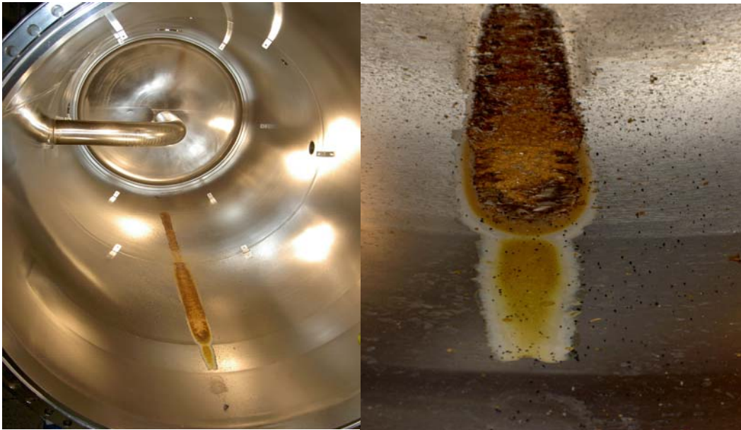
Fig. 3: View into the TIMO test vessel and the deposits at the bottom of the vessel.
