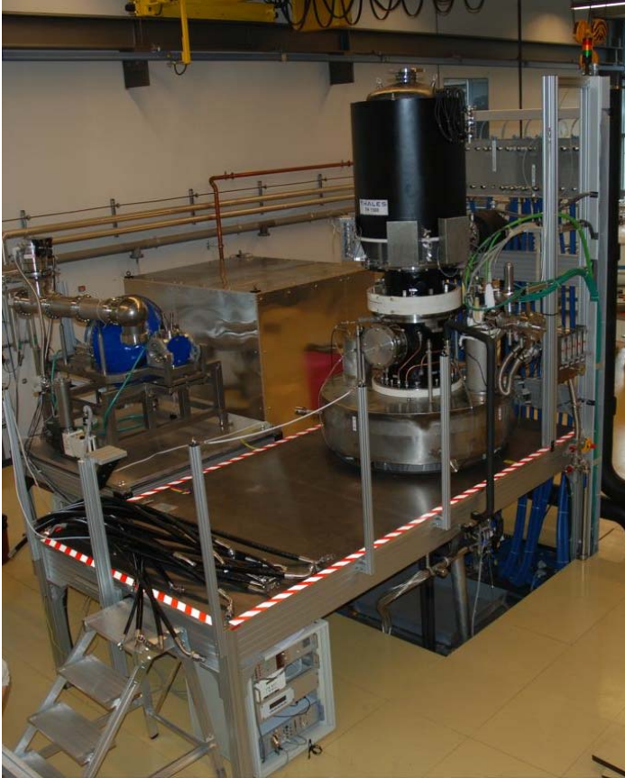
Fig. 1: Photography of the first industrial prototype of the 2 MW, CW, 170 GHz coaxial cavity gyrotron (fabricated by Thales ED) installed in the SC magnet at CRPP Lausanne.
