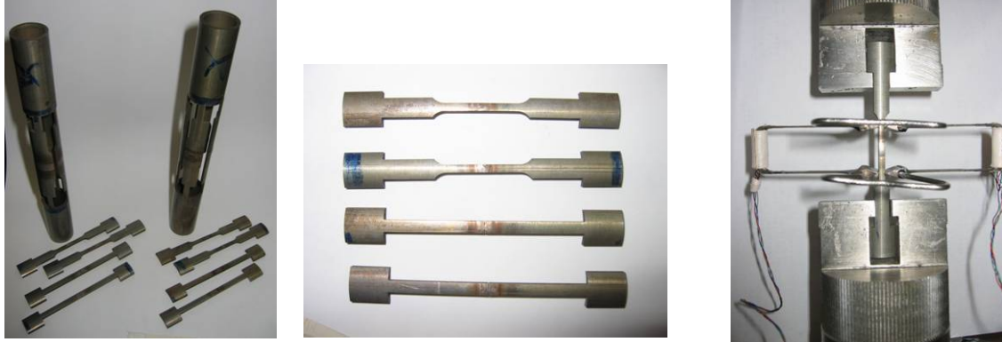
Fig. 3: Welded Dipole conduit material, the obtained specimen made by EDM and installed in the test facility.
