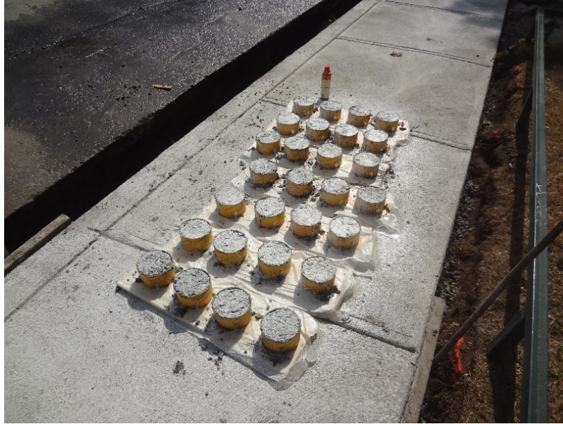
Figure 3.3 Project A; samples provided form walkway concrete casting project.
