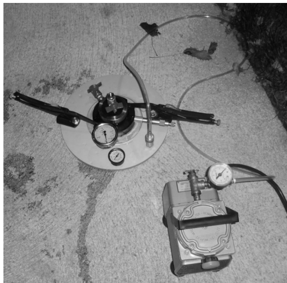
Figure 3.12 In-situ water absorption measurement.
