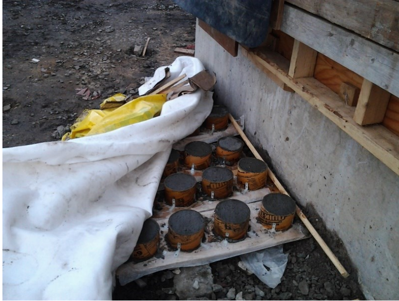
Figure 3.6 Project B; samples provided from the bridge construction project.
