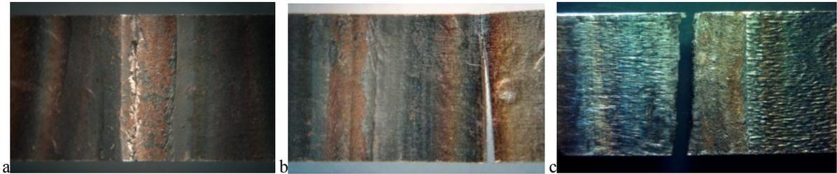
Fig. 9. Fracture location for PAW fatigue testing samples: (a) MS; (b) MB; (c) ZRG.
