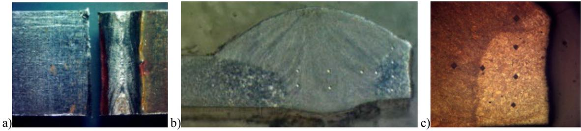
Fig. 8. Fracture location for GMAW fatigue tested samples.
