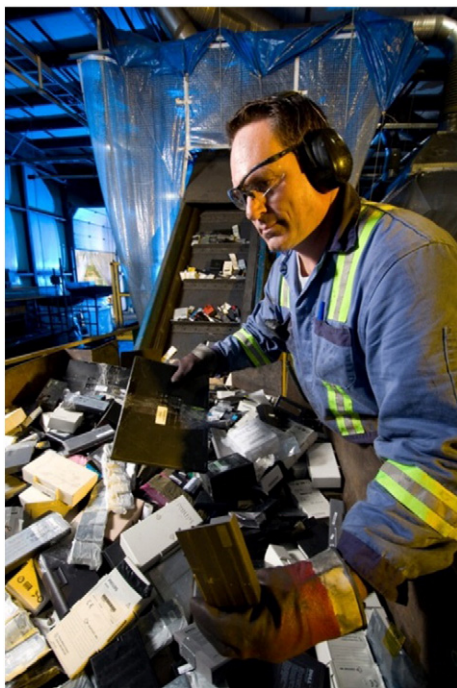
Fig. 4. Hand-sorting of Ni–MH consumer batteries. (Courtesy of Kinsbursky Brothers, Inc.)
