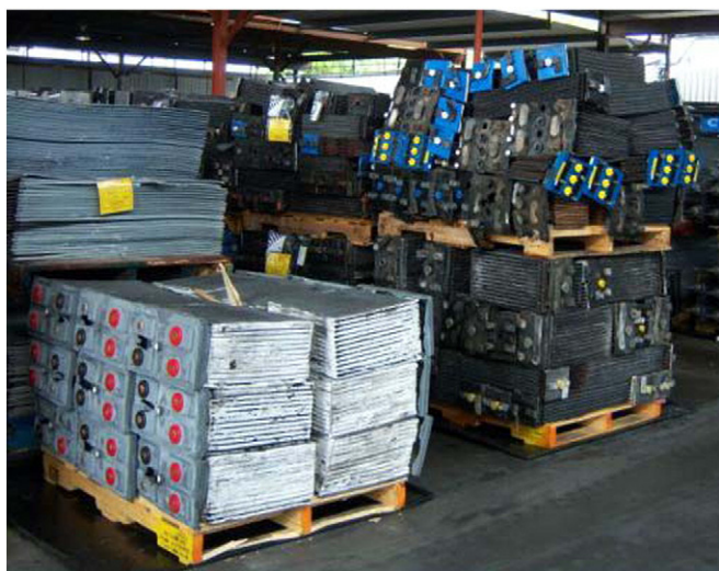
Fig. 3. Lead–acid battery cases and plates after separation.
