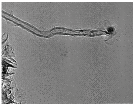
Fig.9: TEM image of the CNT grown in the sample holder wall with the particle of Fe on which has nucleated. Esc. 50nm. (Devaux and Vergnat 2008)
