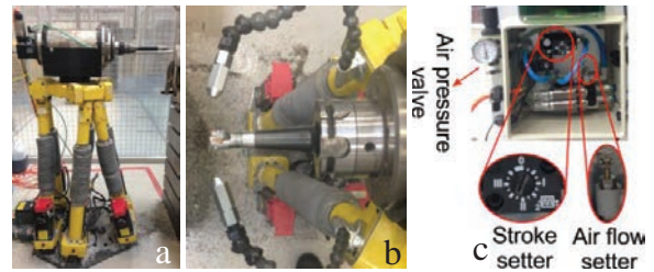
Fig. 1 MQL fitted robotic machining unit. (a) Spindle retrofitted mobile machining (b) MQL mist unit (c) MQL nozzles.
