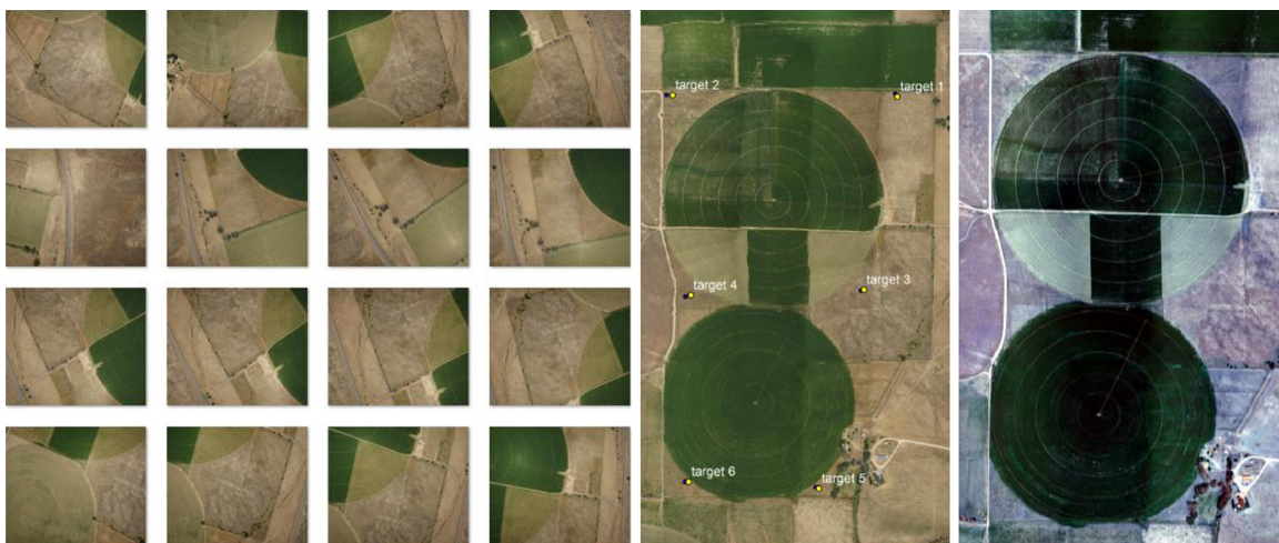
Fig. 4. Raw natural color images from the UAS(left); accurate orthorectified mosaic image from EnsoMOSAIC (center); radiometric calibration of VIS image (right).
