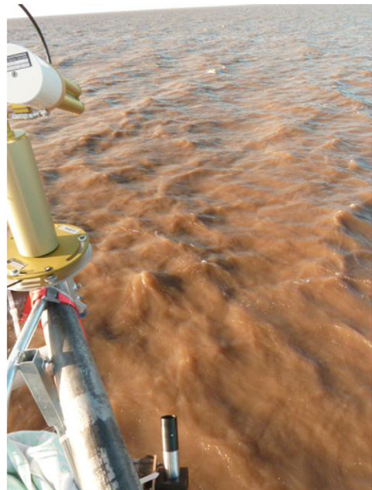
Fig. 10. Photograph of the surface taken in the turbid waters of the Rio de La Plata Estuary for a sun zenith angle of approximately 75^\circ and low wind conditions with typical significant wave height of about 10–20 cm. The sun is to the left of picture and in the foreground radiometer systems are visible. Darkened areas of wave shadowing are clearly visible to the right of the larger wave crests.
