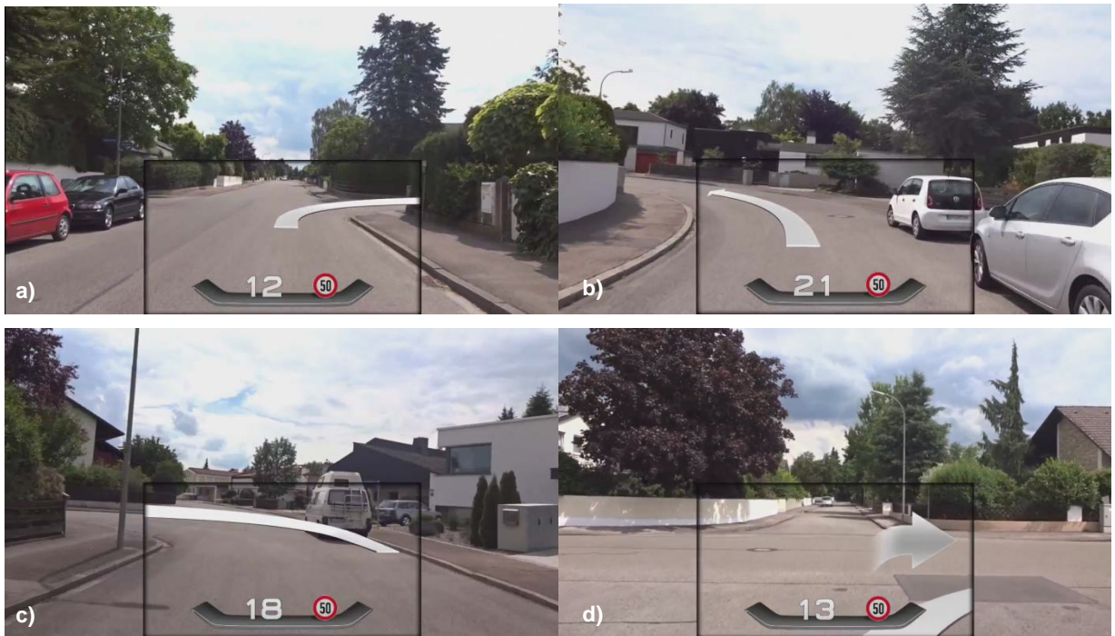
Fig. 3.Arrow concept with the four different design variations: (a) cut-off, (b) no cut-off, (c)tilt, (d) 2D.
