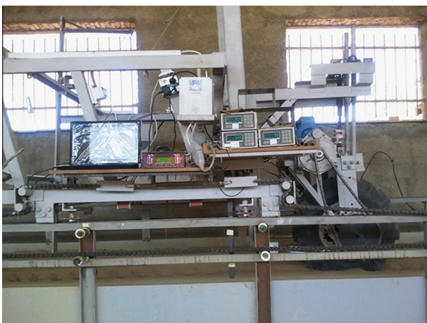
Fig. 1 – The general soil bin facility used for the experiments.
