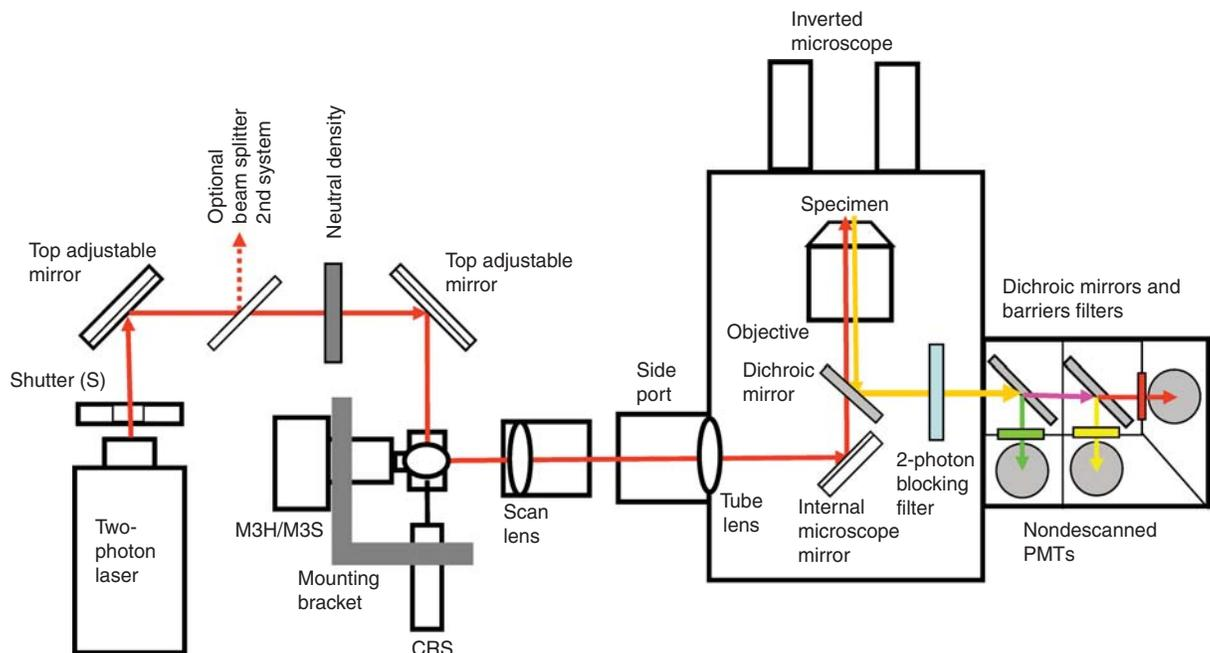
**FIGURE 7.** Basic elements of a two-photon microscope. PMTs detectors do not require pinholes or focused images and are located immediately below the objective. The design is for the most part similar to that of the one-photon laser scanning confocal microscope; see Figure 4.
