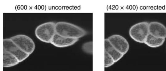
**FIGURE 6.** Images collected with a resonant scanner. *Left* image shows distortion resulting from the slowing of the scan toward the image edges. *Right* image shows the same image after correction that linearizes the scan rate to remove edge distortion.
