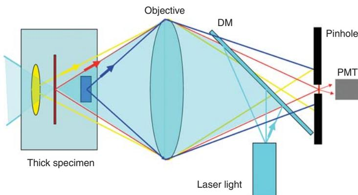
**FIGURE 3.** Principle of operation of a laser scanning confocal microscope. Laser light is focused on the thick specimen by reflection from the dichroic mirror (DM) and the objective lens. The laser excites fluorescence throughout the specimen that passes through the DM and is focused onto the image plane. A pinhole only allows light from the confocal plane of the specimen to reach the photomultiplier tube (PMT).
