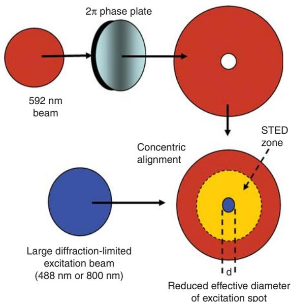
**FIGURE 10.** Creation of reduced excitation spot for STED microscopy. The STED (592-nm) laser beam (red) is shaped by a  $2\pi$  phase plate into a doughnut and concentrically overlaid with the 488-nm excitation laser (blue). The process of STED occurs in the yellow zone to reduce the zone of fluorescence. Increased STED laser power decreases the diameter,  $d$ , of the excitation spot.
