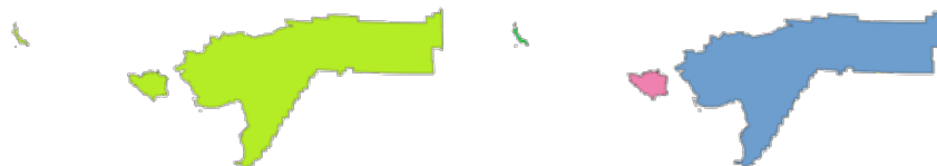
Fig. 25.78: Left the multipart source layer and right the single part output result
