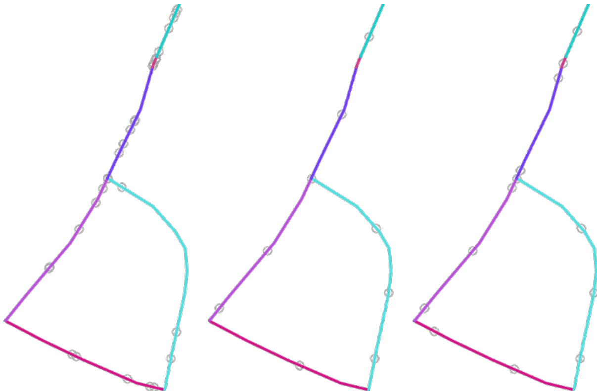
Fig. 25.43: Five points per line feature, left : min. distances = 0, middle : min.distances != 0, right : min. distance != 0, global min. distance = 0
