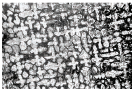
Fig. 2. Photograph showing the primary dendrite spacing in a Ni-based superalloy single crystal obtained by the Bridgman technique with seed. The crystal growth rate was 6 mm/min and the length of the single crystal was 6.36 cm. The photograph was taken at 2 cm from the seed with a magnification of \times 24 .
