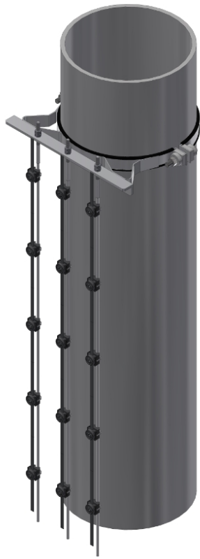
LED-Dot on stainless clip with stainless steel bracket fixed on twin ropes \varnothing 2,0mm and pipe clamp
