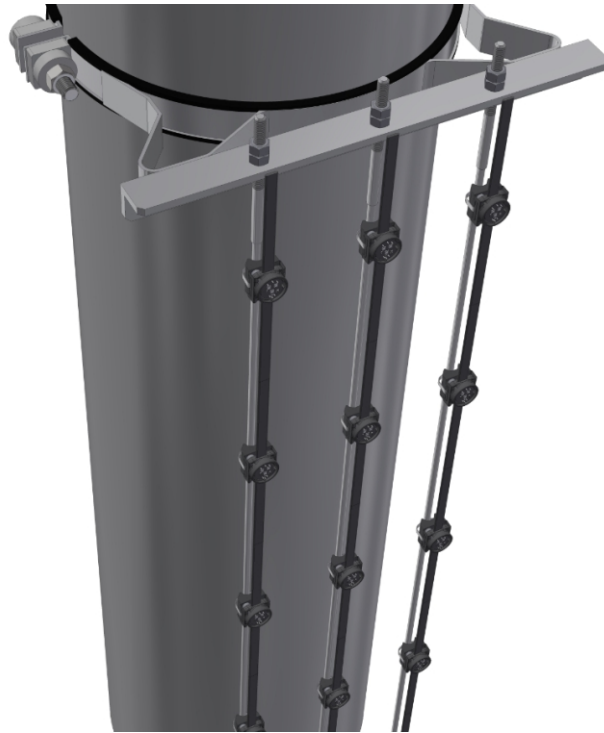
LED-Dot on stainless clip with stainless steel bracket fixed on twin ropes \varnothing 2,0mm and pipe clamp
