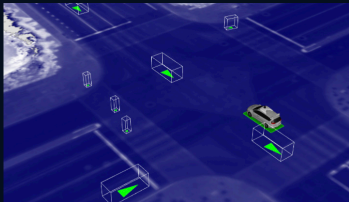
↑ To make a scene more complex, we can add vehicles, pedestrians and cyclists that never existed in the original scene.
