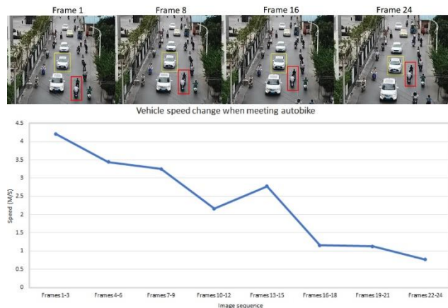
Figure 4: Example for vehicle speed change due to motorbike approaching.
