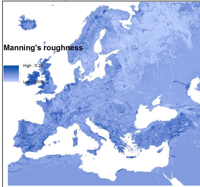
Figure 3-8: Manning's surface roughness at 5km resolution
