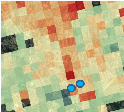
Figure 48- Intensive Energy Consumption Management System (SGIE) plant and potential waste heat consumers in vicinity.
