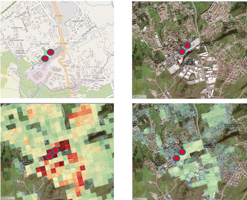
Figure 37- Intensive Energy Consumption Management System (SGCIE) plants in Cabra Figa Industrial Zone and potential waste heat consumers in vicinity
