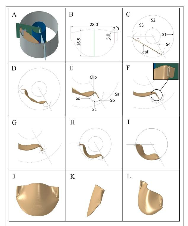
Figure 2, A: Isometric view of the leaflet manipulation system, B: Leaflet geometry the units of which are millimetres, nodes sets X and Y are highlighted in red, a plane of symmetry is highlighted in green, C-I: Depicting the manipulation of the leaflets, J: final geometry rear view, K: final geometry side view, L: final geometry isometric view.
