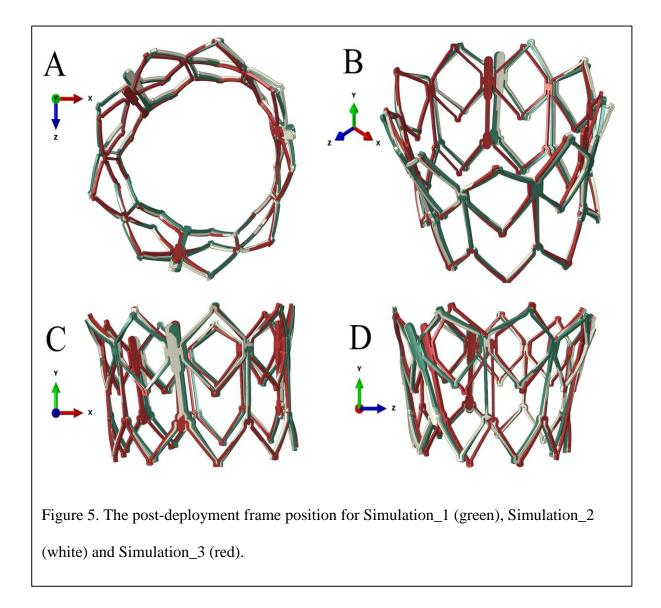
Comparing Simulation\_2 with Simulation\_3 (ANPD=0.0956mm), it is clear that a larger discrepancy is associated with the clips. This resulted from the constraint applied to the clips to construct the model. Coupling constraints were applied to the clips, which are completely rigid. However, in reality, the clips would be stitched to the frame resulting in a more flexible structure.
