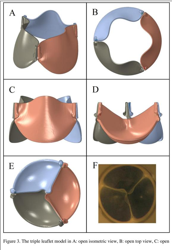
Figure 3. The triple leaflet model in A: open isometric view, B: open top view, C: open side view, D: closed side view, E: closed top view, F: closed top view of an experimental valve.
