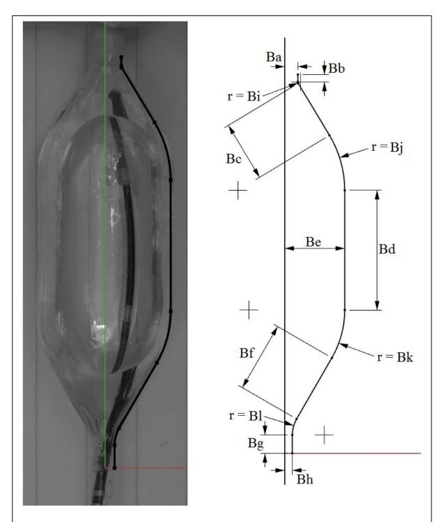
Figure 7. The NovaFlex+ delivery system with the outline of the geometric model overlay (left), the geometric model defined (right).
