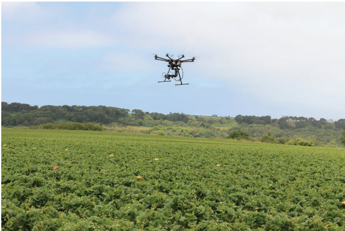
Fig. 4. Airborne remote sensing in California strawberry. Researchers from the University of California Davis obtain canopy reflectance data of arthropod-infested plants with a drone-mounted hyperspectral sensor in a commercial strawberry field.
