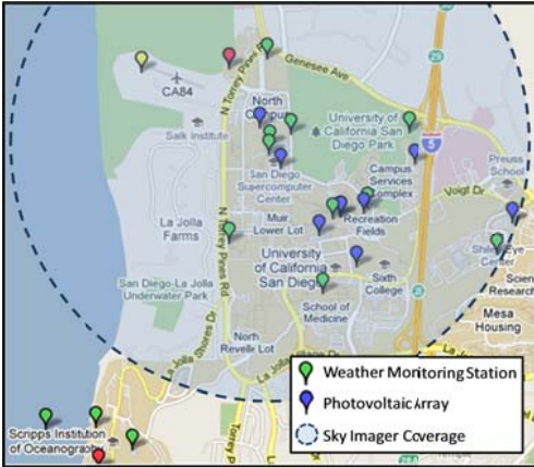
Figure 1: Map of UCSD showing sky imager coverage, weather stations, and PV arrays. The coverage area of the sky imager is a function of cloud base height. The region displayed here has a radius of approximately 2 kilometers which would apply to a cloud base height of 1150 m at a maximum zenith angle of 65°. © Google Maps, 2010
