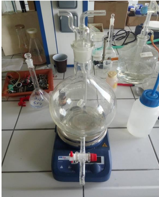
Fig. 1. Stirred recarbonization batch reactor.
