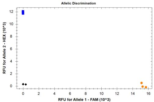
Orange dots are indicative of WT presence (amplification only on FAM channel), **blue** dots are indicative of MUT presence (amplification only on HEX channel) and **black** dots indicates residual non-specific amplification.
