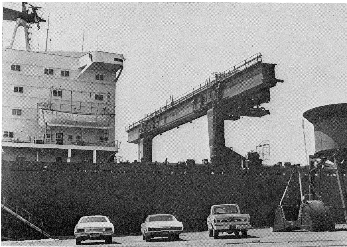
A distinctive feature of Columbus Line ships—the ship-mounted gantry crane which enables them to load and off load their own containers independently of wharf-based cranes.
