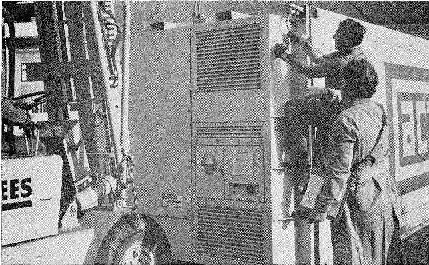
Clip on refrigeration unit being attached to container of perishable cargo. Unit controls temperature inside container.
