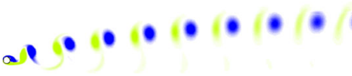
FIGURE 17. (Colour online) A snapshot of vorticity contours at levels between \pm 1 showing the P_1 mode at f_d/f_{St} = 0.80 , A^* = 0.40 . The vortex shedding process is similar to that for the stationary cylinder, except that one vortex is shed on the upstroke of the cylinder, and one on the downstroke of the cylinder, leading to different strength vortices on either side, and hence a non-zero mean lift.
