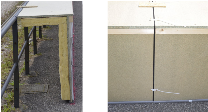
Figure 4: Views of the low-height barrier prototype. Left: cross section. Right: joint system between elements.
