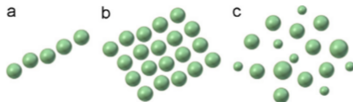
Fig. 4. 3D shape primitives used for assessing terrain traversability. (a) Line, (b) planar patch and (c) cluster of scattered 3D points.
