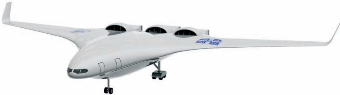
Figure 15.16 ▶ Blended wing body: SAX-40 design
