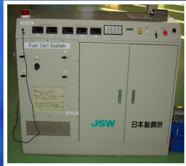
Fuel Cell( PEM Type ) : Output = 900 W
