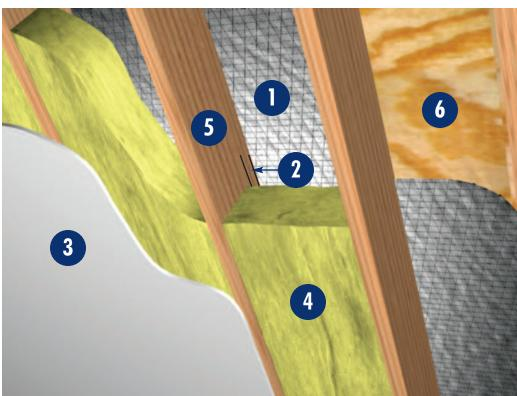
Southern Zone of the USA -With Reflectix® Above the Mass Insulation • R-6.0 Summer & R-2.0 Winter or a Radiant Barrier - Blocks 96% Radiant Heat
