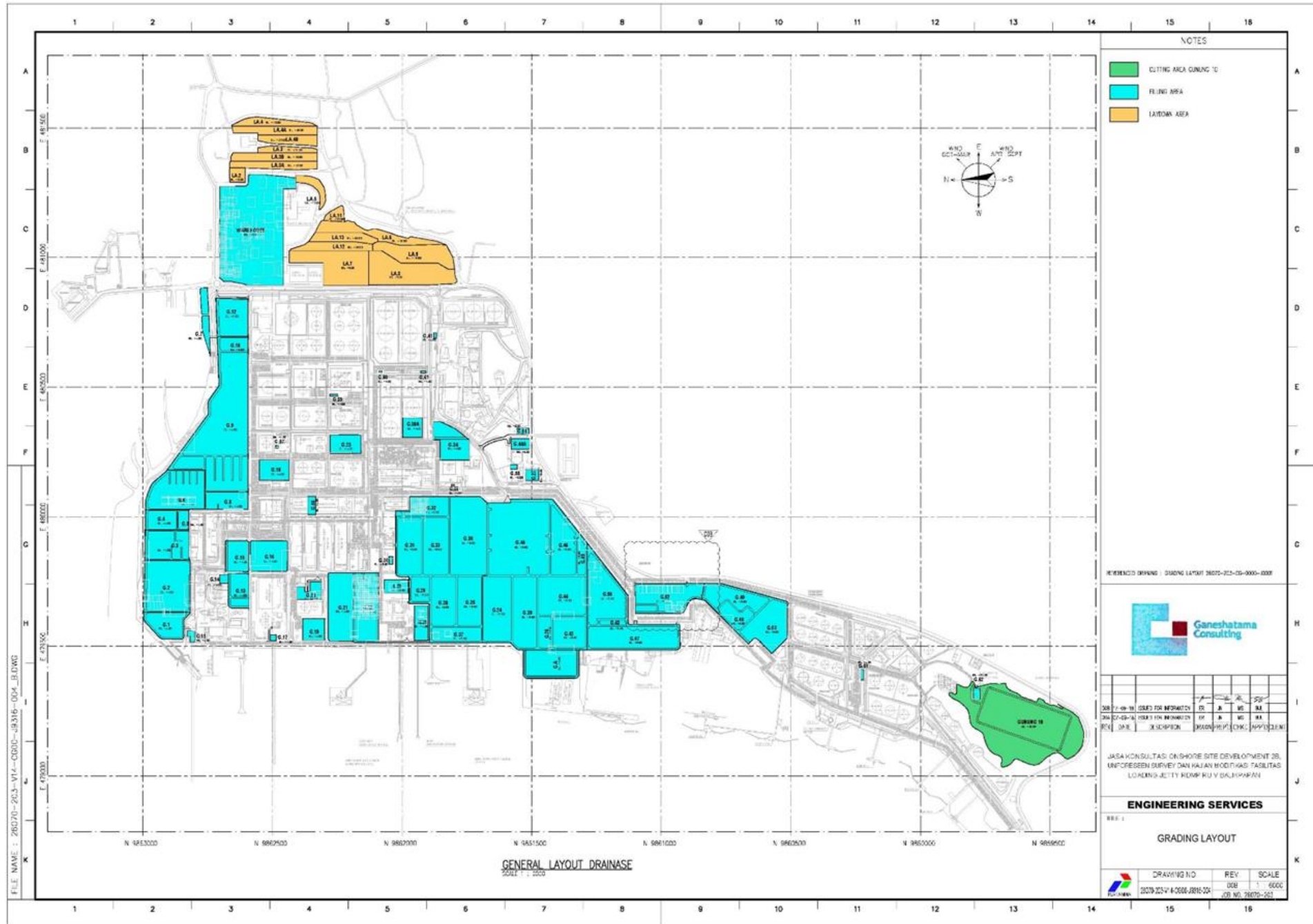
Figure 2.14 Map Location of cut and fill of land materials inside the refinery unit area.
