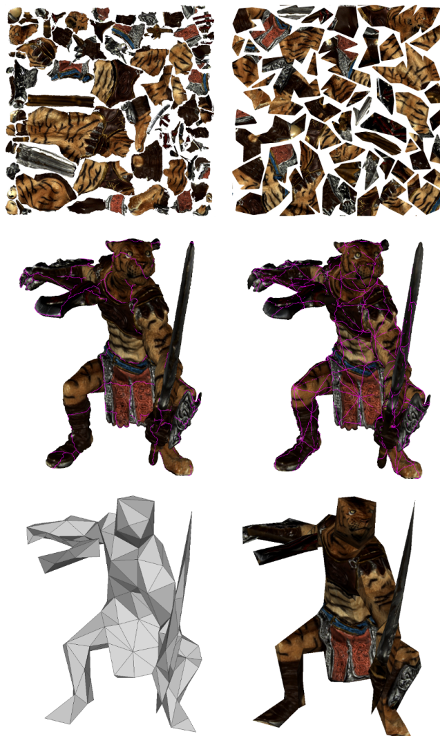
Figure 5: Re-atlasing. Top: input atlas and new atlas. Middle: input seams and seams after re-atlasing via the abstraction mesh. Bottom: abstraction and textured abstraction mesh.
