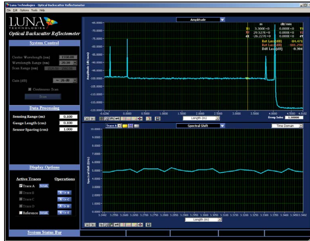
Figure 4-9. Control panel settings for a spectral shift measurement. Note that the Shift Reference is loaded (as indicated by the blue Details button for Trace E ) but not displayed (the Active Traces check box is unchecked for Trace E ).
