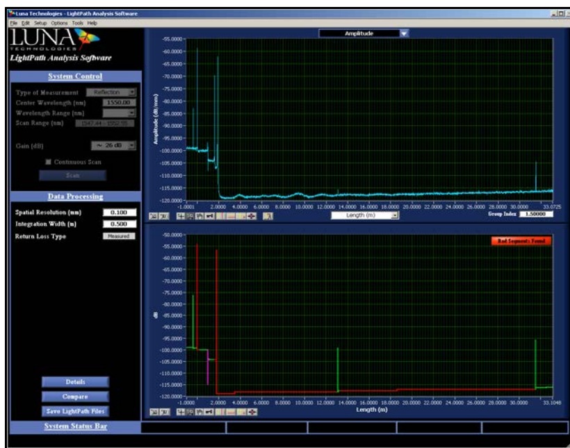
Figure 6-3. Data from the file device1.obr is being compared to the Parameter Configuration File lpa_default_params.ini .
