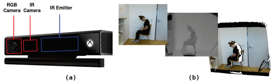
Figure 6. Microsoft Kinect v2 camera with included sensors (a) and illustration of three modalities captured in the the dataset (b): RGB image, depth map, and 3D point cloud.
