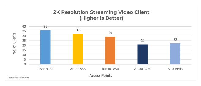
Cisco 9130 was the most capable AP to maintain the most stable and highest number of clients simultaneously while streaming. Aruba AP555 was able to stream up to 32 clients without showing any performance glitches. Ruckus 850 had a decrease of 24 percent in comparison to Cisco 9130. Arista C250 handled up to 21 clients, and Mist AP43 maintained 22 clients – a 71 and 64 percent decrease, respectively, compared to Cisco 9130.
