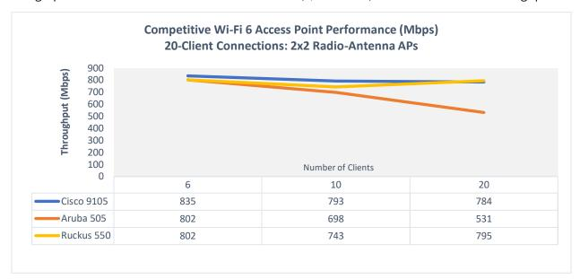
Cisco 9105 had the most consistent and highest performance at 6 and 10 clients in comparison to Aruba 505 and Ruckus 550 APs. Cisco 9105 performance from 6 to 10 clients decreased by only 5 percent, whereas Aruba 505 performance decreased by 13 percent and Ruckus 550 by 7 percent. From 10 to 20 clients, Cisco 9105 only decreased by 1 percent whereas Aruba 505 decreased by 24 percent and although Ruckus 550 performed better, it was not as consistent as Cisco 9105.
