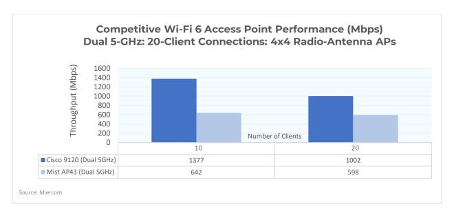
In Dual 5-GHz performance test, Cisco 9120 showed the best results and performed significantly higher than Mist AP43. Cisco 9120 also maintained beyond 1Gbps speed throughout the test. At 10 and 20 clients, Cisco 9120 offered 114 percent and 68 percent better throughput than Mist AP43 respectively.
