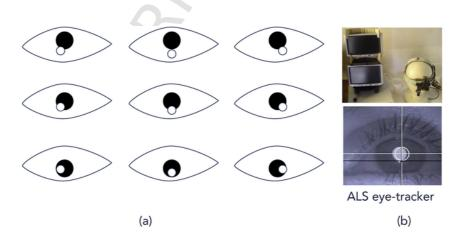
**Fig. 2.** Calibration of an eye-tracker based on video oculography: (a) Illustration of the pupil movements (black circles) and the quasi-stationary corneal reflections (small white circles) needed to calibrate an eye-tracker whose calibration depends on nine points (ASL eye-tracker); (b) Image of the user's eye taken by the eye-tracking device during system calibration.
