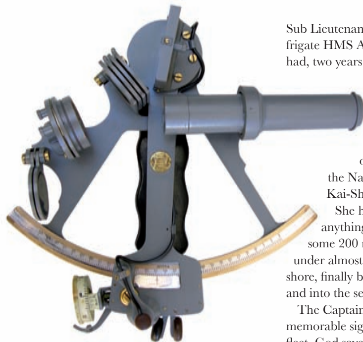
Above: Sextants were used for navigation and comprised both a telescope and protractor for measuring angular distance above the horizon.
