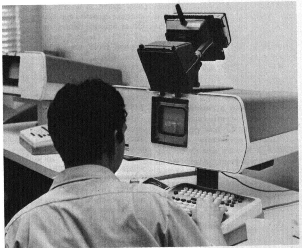
A camera is mounted on the graphics display terminal, connected to the UCLA computer, for permanent recording purposes. (Photo University of California, Los Angeles)
