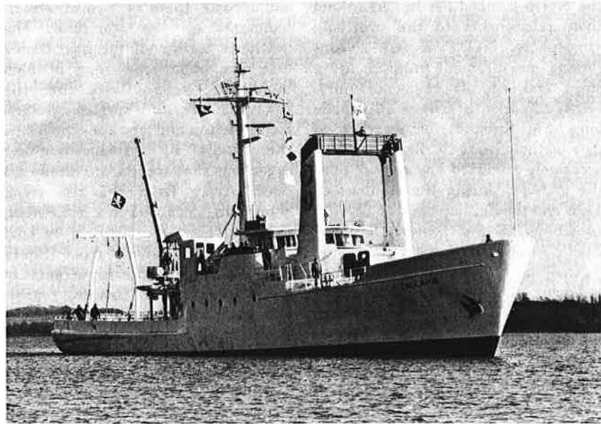
Modern research ship. R/V ENDEAVOR , the third of three new oceanographic vessels, was added to the Nation's academic fleet in 1976. This 177-foot-long OCEANUS -class ship, designed expressly for research, is being operated by the University of Rhode Island.
