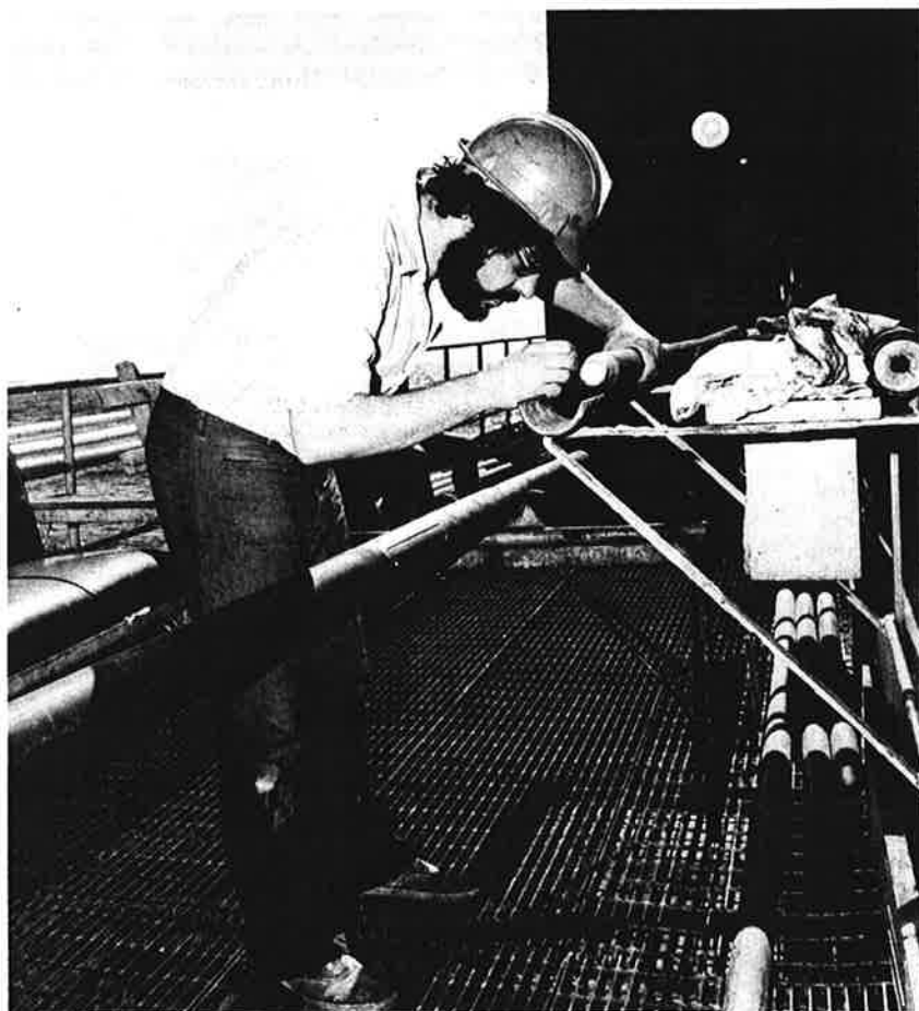
Aboard GLOMAR CHALLENGER. Philip Rabinowitz of Lamont-Doherty Geological Observatory, a co-chief scientist on Leg 45 of the Deep Sea Drilling Project, inspects a downhole hydrophone used to measure sonic characteristics of rocks below the ocean floor. DSDP research in 1976 resulted in new findings about young crustal material and about events associated with the splitting of North America from Europe and Africa.
